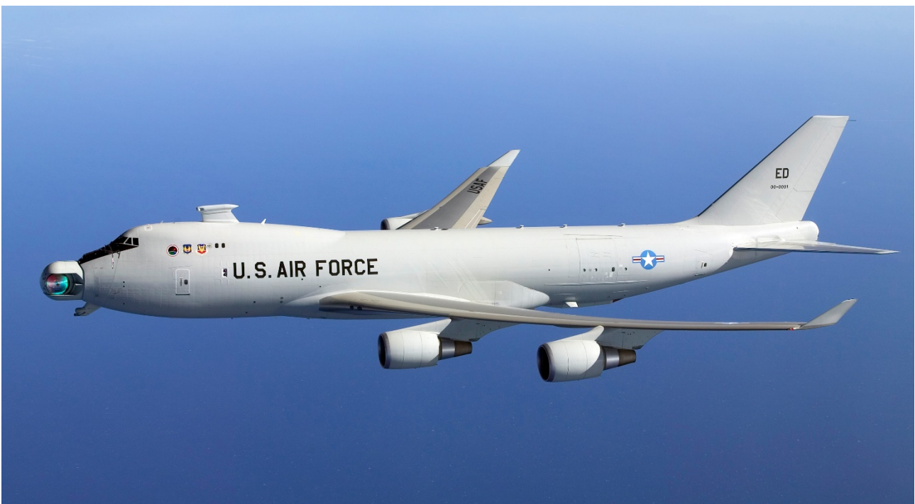
YAL-1 Airborne Laser Test Bed with the mirror visible in the nose [US-MDA]
