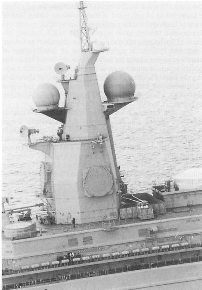
Fig. 8 Octagonal antennae (3) amidships the SSV-33.
