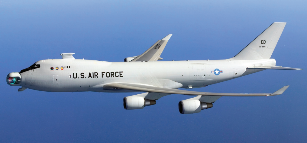
Links: YAL-1 Airborne Laser Test Bed met de spiegel zichtbaar in de neus [US-MDA]. Rechts: MIRACL Mid-Infrared Advanced Chemical Laser Beam Director. [Wikipedia]
