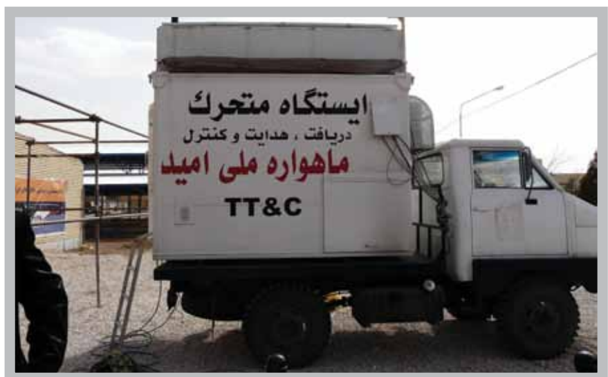
Telemetry Tracking & Control bus. [M van Eijkeren]
