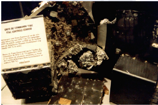
OTS 1 fragment, recovered from the Ocean after the Delta rocket failed to put the satellite in orbit. [Skynet.be]
